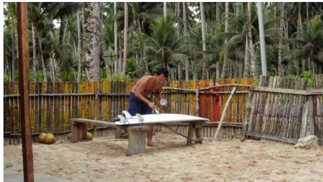
Figure 26: Aprianto applies the resin to the board, before leaving it to dry out in the sun
