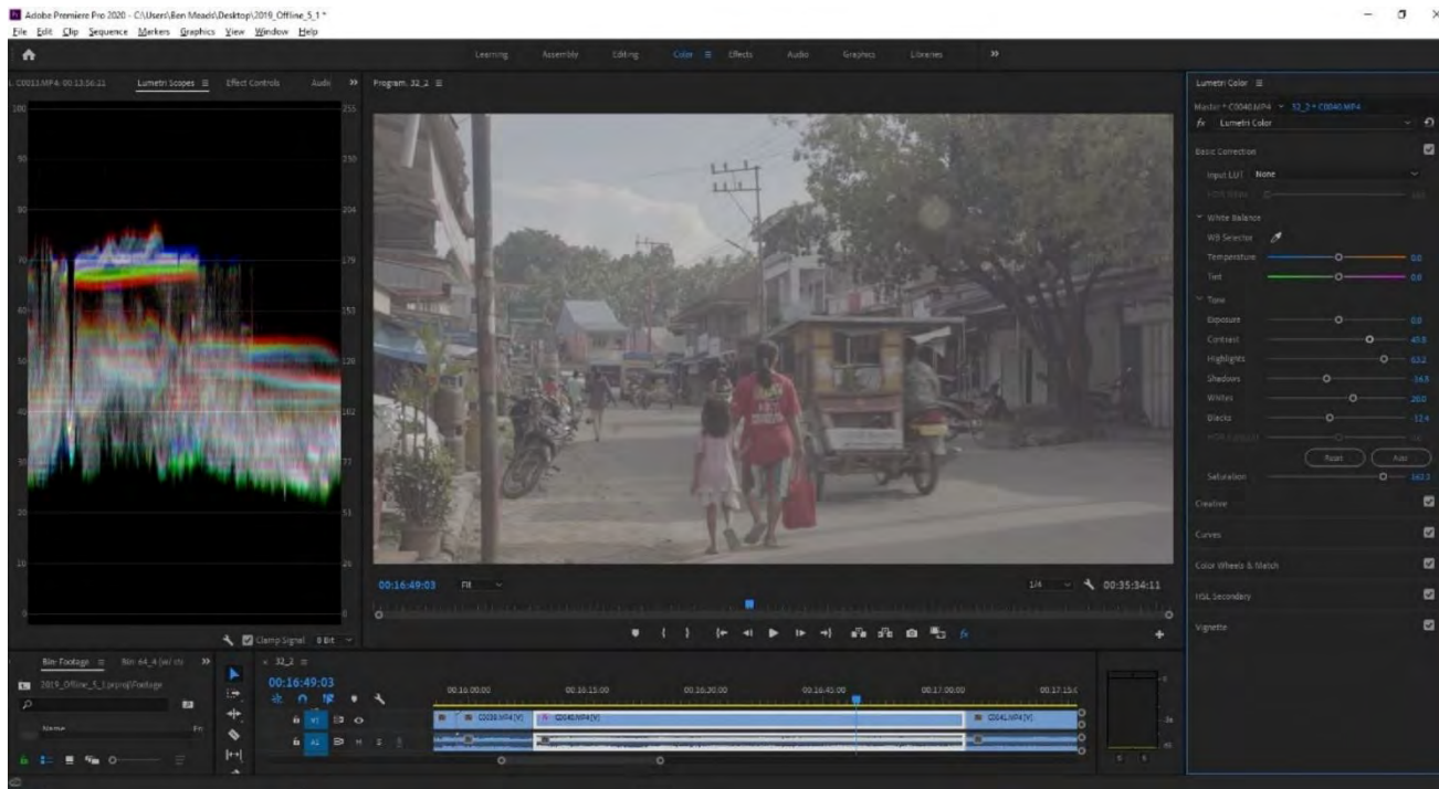
Figure 69: In 'log' - the greyed-out image lacks contrast and saturation, but all of the information is there, waiting in the middle of the compressed histogram
