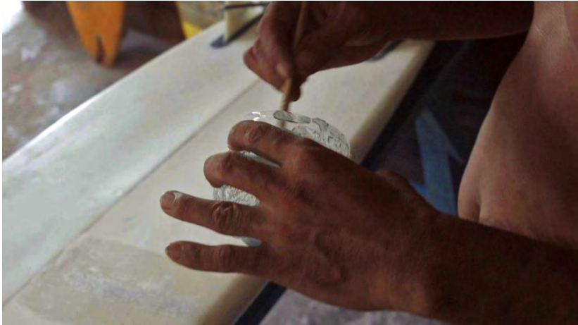
Figure 22: Aprianto mixes resin to seal up a 'ding' on the surfboard
