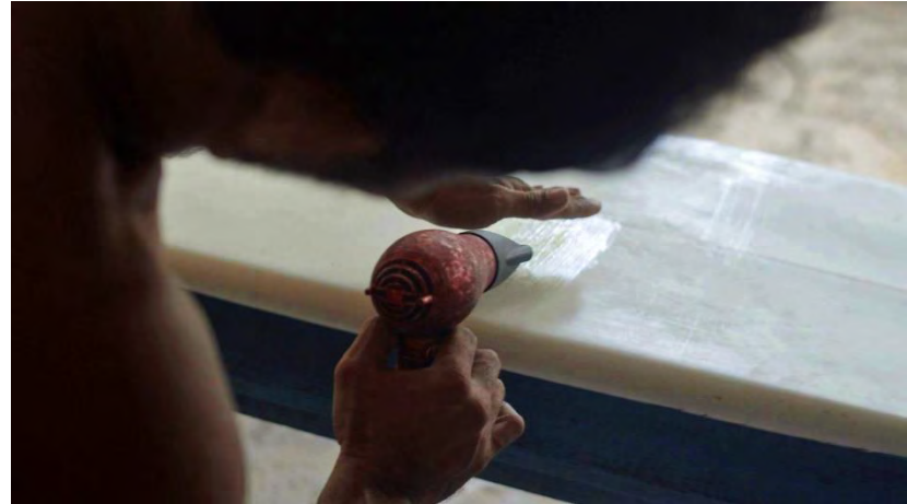
Figure 25: Drying the resin application with a hairdryer
